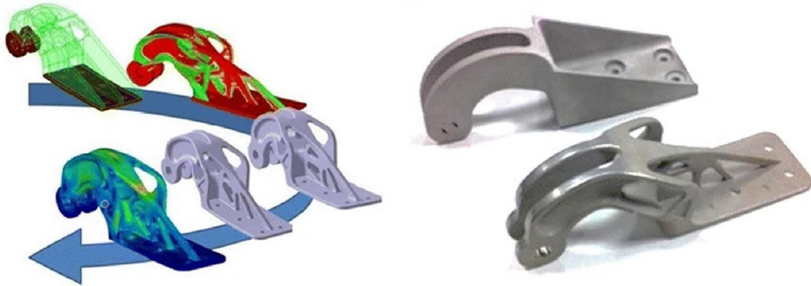
Fig. 1. TO and AM of Airbus A320 nacelle hinge bracket. Left: TO design process. Right: Original bracket (top) and final TO optimized design (bottom) . Original steel bracket = 918 g; TO and AM bracket in Ti6Al4V = 326 g.(M. Lang,2019)
